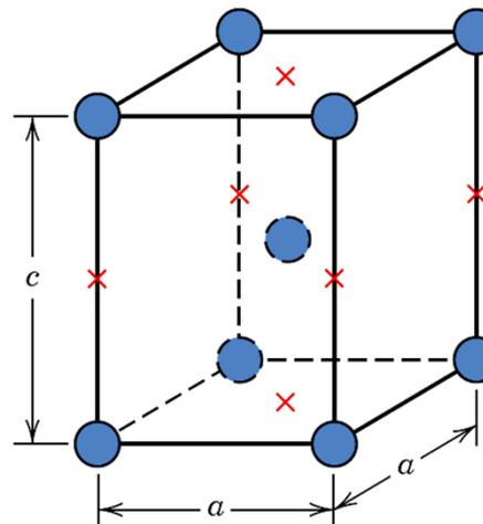
**Body-centered tetragonal unit cell** ( $c > a$ ) for martensitic steel structure, showing **iron atoms (circles)** and sites occupied by **carbon atoms (Xs)**.
