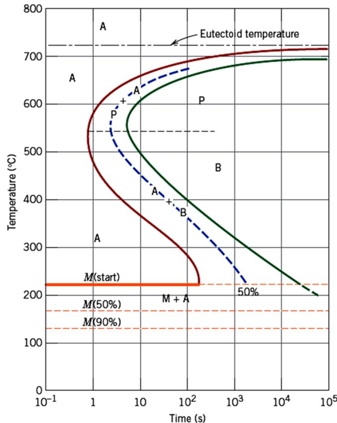
TTT diagram for **unalloyed eutectoid steel (0.8% C)**
