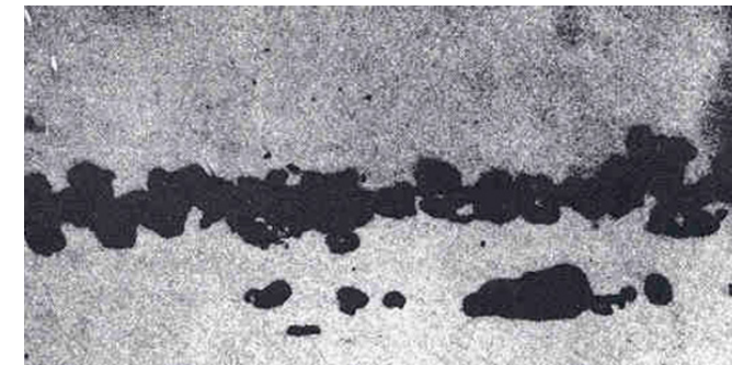
Brittle inclusions (black) during hot rolling of a heat-resisting steel
