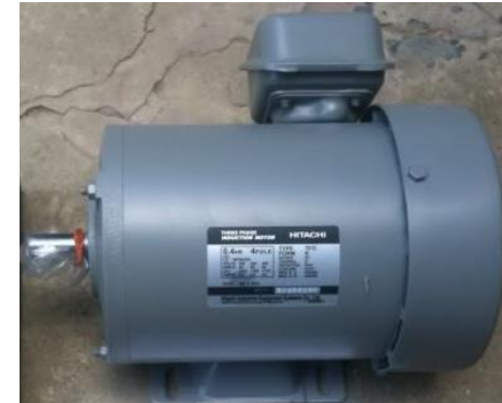
Option 2: use a small three-phase induction motor and observe its rotation direction
