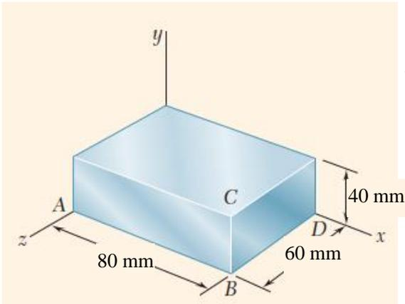
Determine the change in volume  $\Delta V$  of the steel block shown in Figure, when it is subjected to the hydrostatic pressure  $p=180$  MPa. Use  $E = 200$  GPa and  $\nu=0.29$ .
