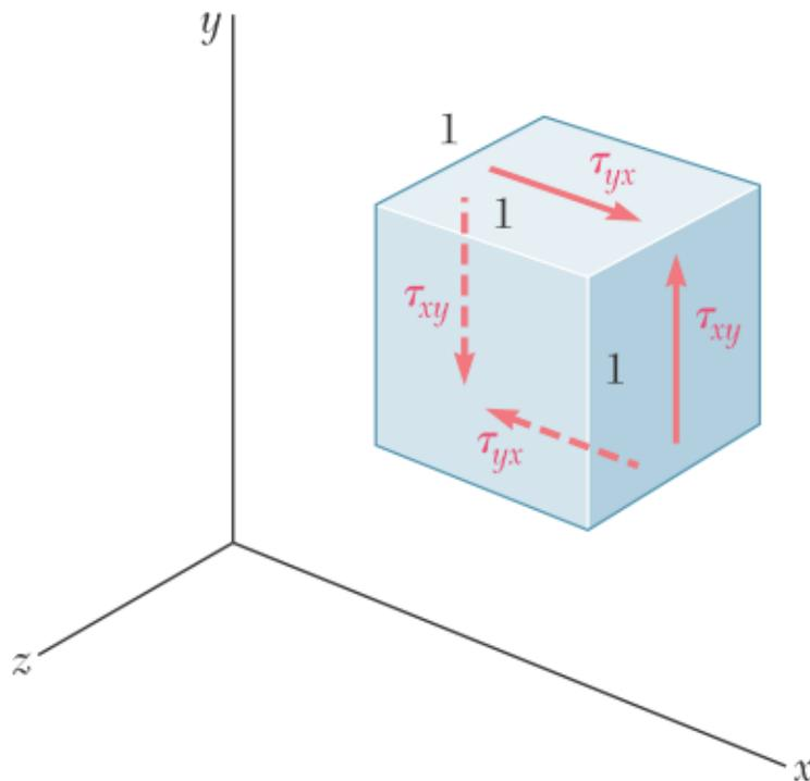
Unit cubic element subjected to shearing stress.
