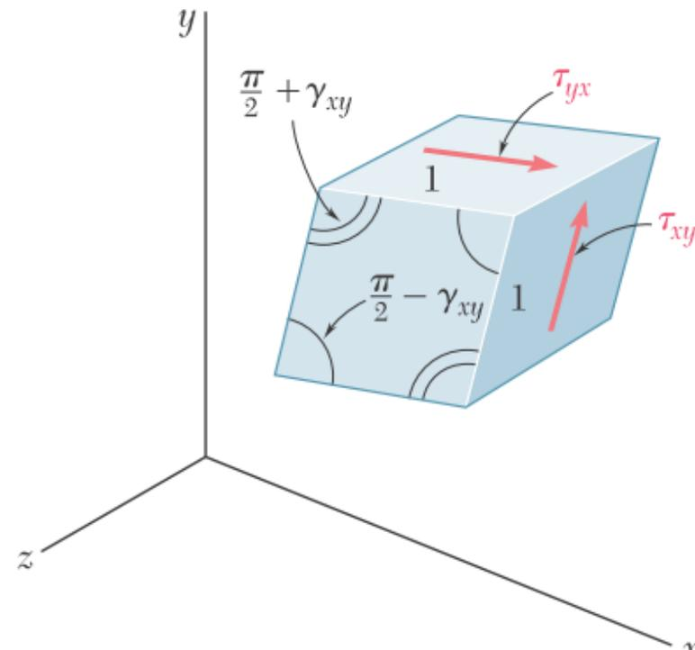
Deformation of unit cubic element due to shearing stress.
