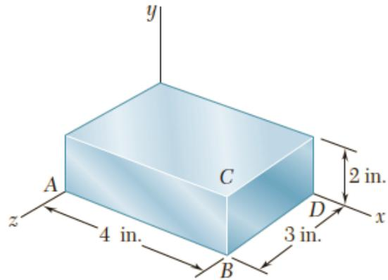
The steel block shown (Fig. 2.34) is subjected to a uniform pressure on all its faces. Knowing that the change in length of edge AB is  $-1.2 \times 10^{-3}$  in., determine (a) the change in length of the other two edges and (b) the pressure  $p$  applied to the faces of the block. Assume  $E = 29 \times 10^6$  psi and  $\nu = 0.29$ .
