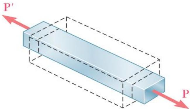
In all engineering materials, the elongation produced by an axial tensile force  $P$  in the direction of the force is accompanied by a contraction in any transverse direction.
