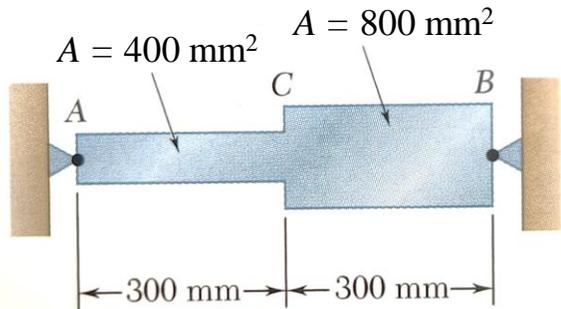
Expressing that the total deformation of the bar must be zero as a result of the imposed constraints, write
