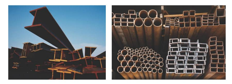
• The longitudinal shear and horizontal shear per unit length (shear flow) are used in this section to calculate both the shear flow and the average shearing stress in thin-walled members such as the flanges of wide-flange beams, box beams, or the walls of structural tubes
