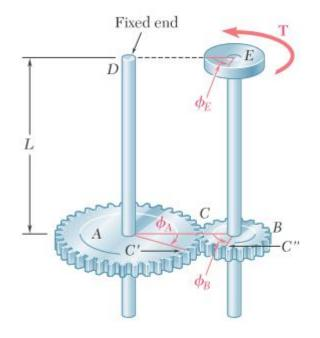
Let's consider shaft BE which both ends are free to rotate, so the angle of twist of the shaft is  $\phi_{E/B}$  through which end E rotates with respect to end B.
