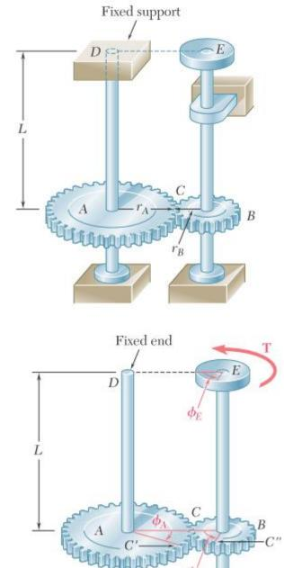
What torque should be applied to the end of the shaft to produce a twist of  $2^{\circ}$ ? Use the value G = 77 GPa for the modulus of rigidity of steel.
