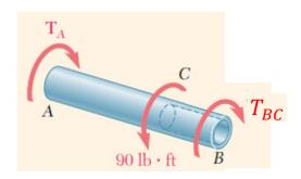
$T_A + T_B = 90 \text{ lb-ft}$   $T_{AC} - T_A = 0 \rightarrow T_{AC} = T_A$   $90 - T_A - T_{BC} = 0 \rightarrow T_{BC} = 90 - T_A$
