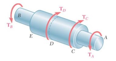
• For shaft AB shown in figure, four different parts should be considered: AC, CD, DE, and EB. The total angle of twist of the shaft (i.e., the angle through which end A rotates with respect to end B) is obtained by algebraically adding the angles of twist of each component part. Using the internal torque  $T_i$ , length  $L_i$ , cross-sectional polar moment of inertia  $J_i$ , and modulus of rigidity  $G_i$ , corresponding to part i, the total angle of twist of the shaft is
