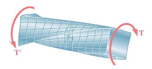
• Equations used to define the distributions of strain and stress in an elastic circular shaft cannot be used for noncircular members. For example, it would be wrong to assume that the shearing stress in the cross section of a square bar varies linearly with the distance from the axis of the bar and is therefore largest at the corners of the cross section. The shearing stress is actually zero at these points.
