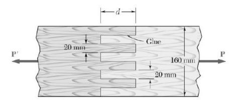
Seven surfaces carry the total load  $P = 7.6 \text{ kN} = 7.6 \times 10^3$ .
