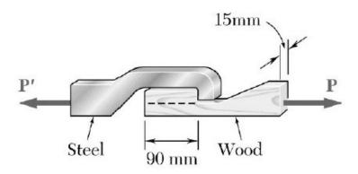
Area being sheared:  $A = 90 \text{ mm} \times 15 \text{ mm} = 1350 \text{ mm}^2 = 1350 \times 10^{-6} \text{m}^2$
