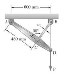
Link BC is 6 mm thick and is made of a steel with a 450-MPa ultimate strength in tension. What should be its width w if the structure shown is being designed to support a 20-kN load P with a factor of safety of 3?
