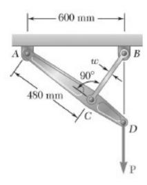
Link BC is 6 mm thick, has a width w = 25 mm, and is made of a steel with a 480-MPa ultimate strength in tension. What was the safety factor used if the structure shown was designed to support a 16-kN load P?
