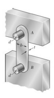
Link AB, of width b = 50 mm and thickness t = 6 mm, is used to support the end of a horizontal beam. Knowing that the average normal stress in the link is -140 MPa, and that the average shearing stress in each of the two pins is 80 MPa, determine (a) the diameter d of the pins, (b) the average bearing stress in the link.
