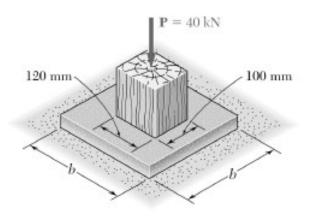
A 40-kN axial load is applied to a short wooden post that is supported by a concrete footing resting on undisturbed soil. Determine (a) the maximum bearing stress on the concrete footing, (b) the size of the footing for which the average bearing stress in the soil is 145 kPa.
