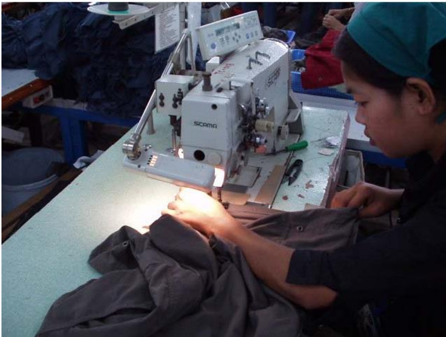
Figure 3: For close-up work it is essential to have local lighting where the light shines directly on the task and not into the workers' eyes.
