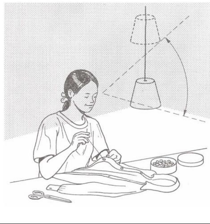
Figure 5: The correct positioning of lights avoids discomfort glare but care should be taken to avoid shadows on the working area. Look at the worker on the right – the light is almost behind her head so that she is working in her own shadow.
