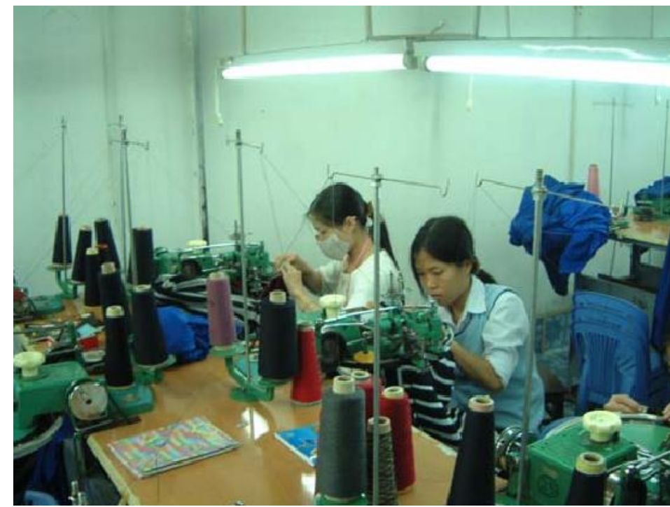
Figure 6: Avoid polished surfaces – use matt finishes or move the work position by 90 degrees to the right or left to stop reflected glare .
