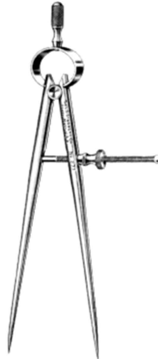
Caliper used as divider
