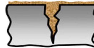
1 Crack filled with dirt
