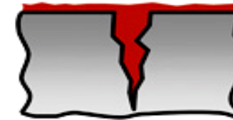
3 Application of penetrant
