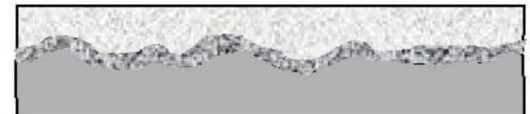
(d) Finally, the bond is formed ideally as a perfect interface boundary.
