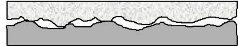
(a) Hard ceramic and ductile metal surfaces come into contact at asperity tips.
