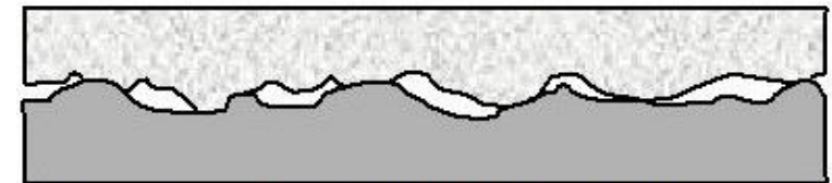
(b) Ceramic asperities indent the metal surface that yields plastically under large local stress.
