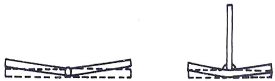
a. Transverse shrinkage in a butt weld. b. Longitudinal shrinkage in a butt weld.
