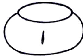
(a) Surface cracks (in upsetting or rolling)
