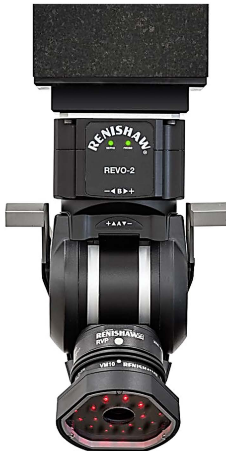
RVP Vision Probe (5-axis non-contact measurement)
