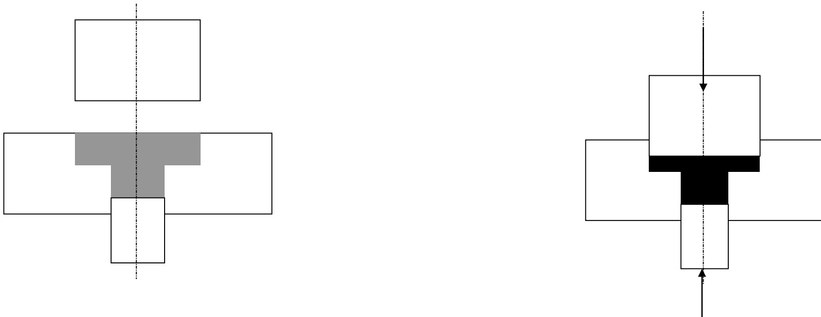
Fig. 1.10 Pressing, the conventional method of compacting metal powders in PM
