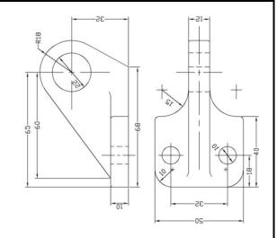
Draw the front and top views add left-side view of the object with scale 1:1
