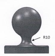
Draw an arc of a given radius tangent to an arc and a line
