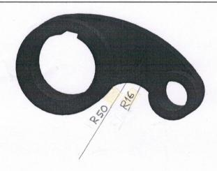
Draw a concave arc and a convex arc of given radii tangent to two arcs.
