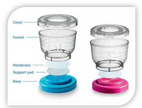
**3-** Take 50 mL of water sample and pour into funnel without filter paper to make a trial run to wet the surface of coarse filter. Run the vacuum pump and open the tap of funnel.
