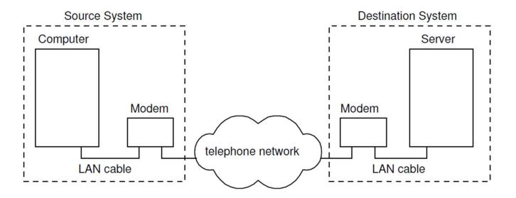
Source and transmitter are separate devices (similar at destination)
