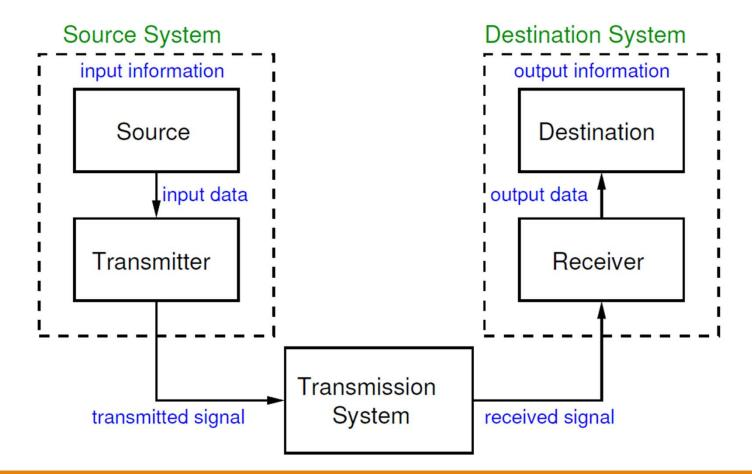
A Model of Communication Systems Aim: Transfer information from source to destination **Source:** Device that generates data to be transmitted **Transmitter:** Converts data from source into transmittable signals **Transmission System:** Carries data from source to destination > Maybe simple as a single link/cable > Or a complex network, e.g. the Internet **Receiver:** Converts received signal into data **Destination:** Takes and uses incoming data
