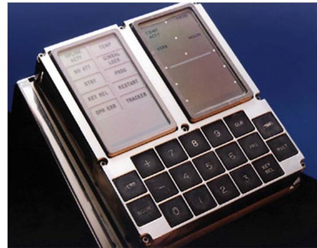
Fig. 2 Apollo Guidance Computer (AGC), was part of the guidance and navigation system used by NASA in the Apollo program for various spaceships.
