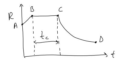
Stage A-B and A'-R: These stages represent a settling down period during which the solid surface conditions come into equilibrium with the drying air.
