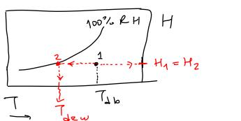
Dry Bulls Temp. (Tob): Temperature measured by a dry thermometer immersed in vapor - gas (air) mixture. It is the T of heated air to be used in drying operation. Équilibrium Moisture Content (X\*): At a given T and P, the moisture content of a moist solid in equilibrium with the gas-vapor mix ture. MC Drying at 502 MC in Trabzon Hzo rema in food in Gaziantep time time MC ٥L Х  $T_3 > T_1 > T_2$  $X_{2}^{*}$  $\times_1^*$ 73  $\times_3^*$ @ Rf %RH (i.e., aw) of surrounding air = aw of food
