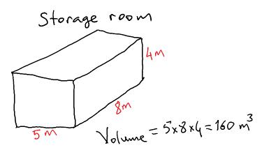
We need to calculate the floor separately from the wall and ceiling, because the temperature difference is different under the floor, so the heat transfer will also be different. Walls and Ceiling
