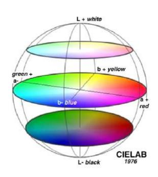
Total Color Difference (TCD): 2 + is calculated from the parameters L, a, b.  $TCD = \sqrt{(L_0 - L)^2 + (a_0 - a)^2 + (b_0 - b)^2}$
