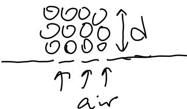
$$t_c = \frac{\rho_s \times \lambda_w \times d \times (X_1 - X_c)}{(T - T_{wb}) \times h}$$
