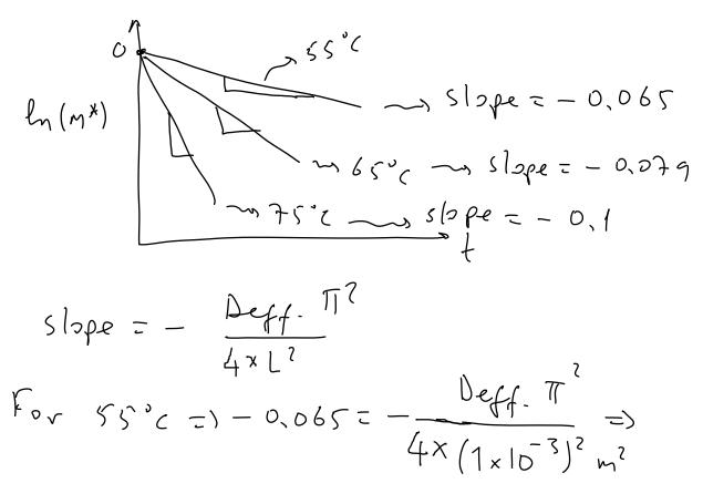
$D_{eff}$  at 55°C = 2.63x10<sup>-8</sup> m<sup>2</sup>/min  $D_{eff}$  at 65°C = 3.2x10<sup>-8</sup> m<sup>2</sup>/min  $D_{eff}$  at 75°C = 4.056x10<sup>-8</sup> m<sup>2</sup>/min
